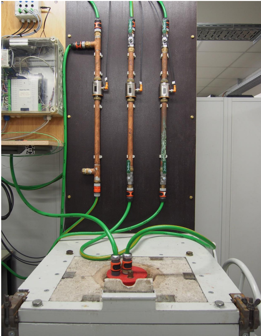
Figure 5: experimental setup. The induction crucible furnace is shown below, including the metal probe and the water-cooling system. On the left side, the Delphin Expert Key 100L, collecting all of the data coming from the setup itself.
